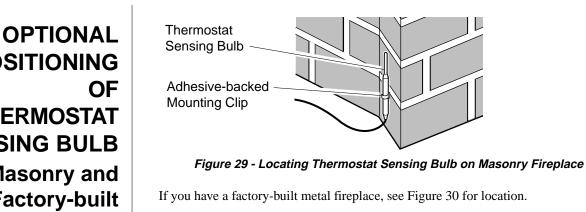
Thermostat Sensing Bulb Adhesive-backed Mounting Clip
